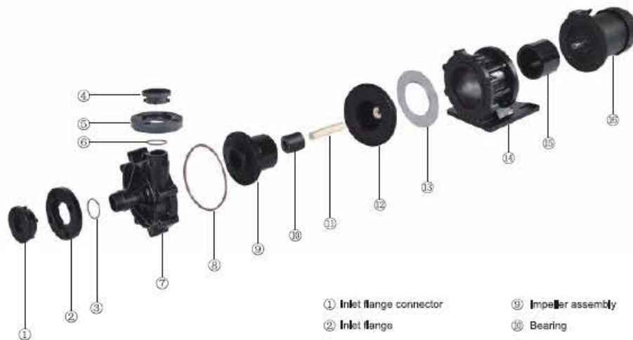
Decomposition diagram of QHX
